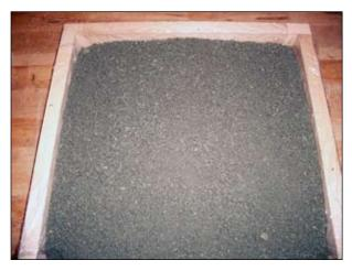
**FIGURE 1.** Cement-coated particles distributed in the form mould.
