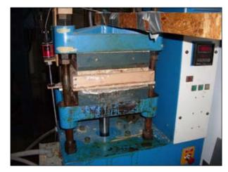
FIGURE 2. Press mat at ambient condition for 24 hours.
