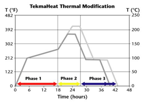
FIGURE 1. Three-phase thermal modification process patented by the Finnish ThermoWood Association.
