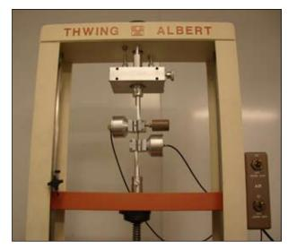
**FIGURE 2.** Preliminary tension test of strips made from wood-plastic composites containing MPB-killed wood.
