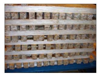
FIGURE 1. Thick MPB strand composite specimens.
