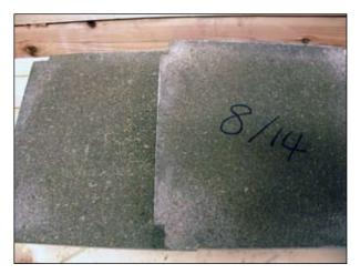
FIGURE 3. The cured cement-bonded particleboards.
