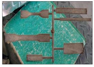
**FIGURE 3.** Set of WPC injection moulding specimens containing MPB-killed wood.
