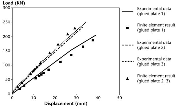
FIGURE 2. Comparison between experimental data and numerical analysis for glued plates.
