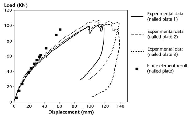
FIGURE 3. Comparison between experimental data and numerical analysis for nailed plates.
