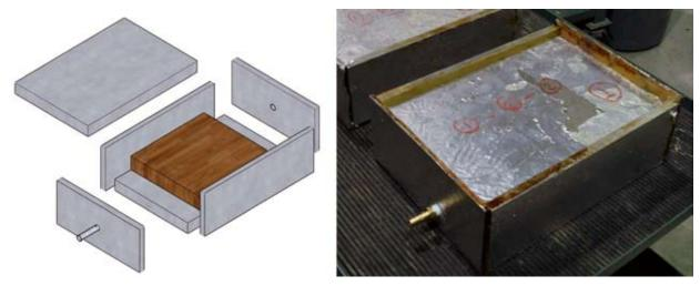
FIGURE 3. Permeability jig design and assembled for testing.
