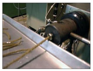
**FIGURE 1.** Extrusion processing of wood-plastic composites.
