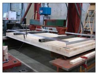
**FIGURE 1.** Bending test of a three-layer cross-laminated MPB wood plate.
