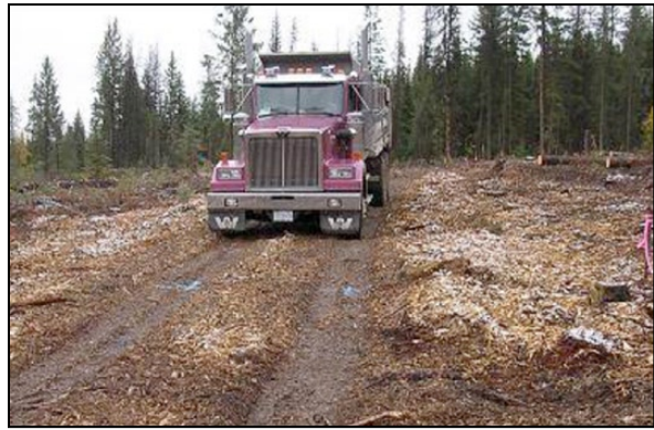
FIGURE 2. Cyclic loading tests of mulched wood road.
