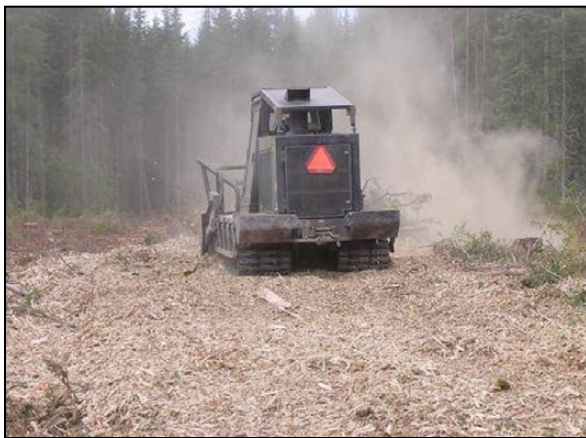
FIGURE 1. Gyro Trac GT-25 mulching windrow of waste material.
