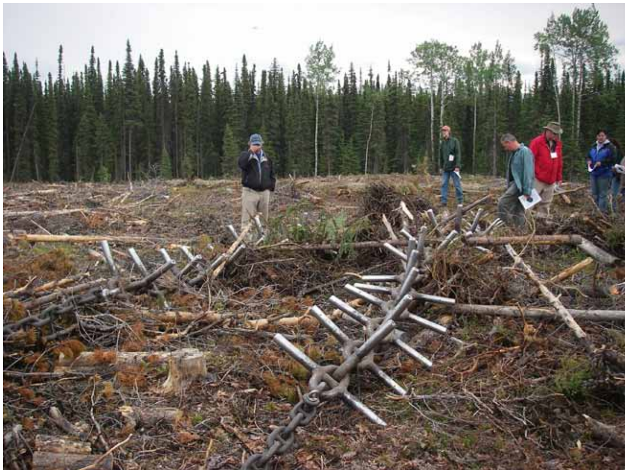
FIGURE 2. Configuration of the drags used by Canadian Forest Products in their Mackenzie Forest District operations (Photo by Alan Wiensczyk).
