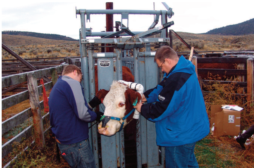
Figure 2. Yoke and harness system used to sample 24-hour enteric methane production
