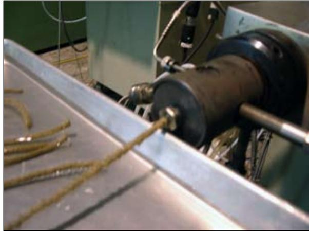
FIGURE 1. Extrusion processing of wood-plastic composites.
