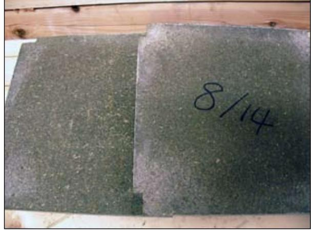
FIGURE 3. The cured cement-bonded particleboards.
