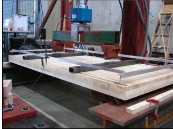
FIGURE 1. Bending test of a three-layer cross-laminated MPB wood plate.
