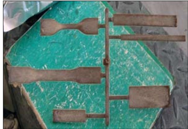
**FIGURE 3.** Set of WPC injection moulding specimens containing MPB-killed wood.
