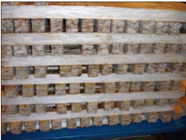
FIGURE 1. Thick MPB strand composite specimens.
