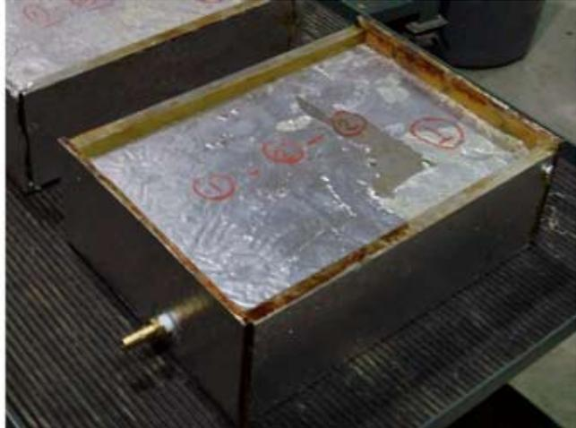
FIGURE 3. Permeability jig design and assembled for testing.
