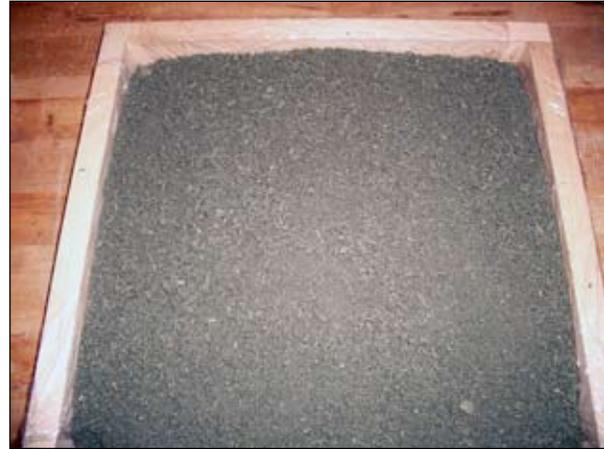
FIGURE 1. Cement-coated particles distributed in the form mould.
